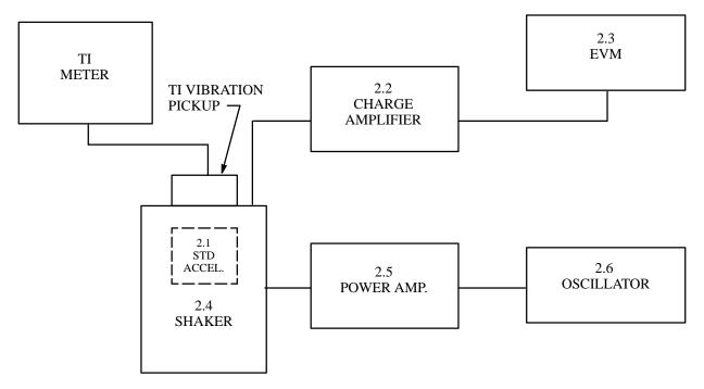
Figure 1. Test Configuration
