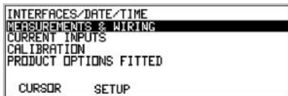
Figure 7. Setup Index screen with MEASUREMENTS & WIRING selected
