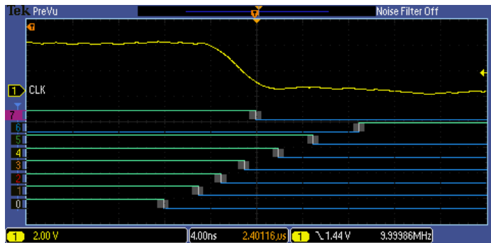
White edges indicate additional information is available by acquiring at a higher sample rate.
